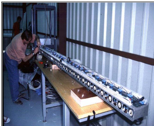
Figure 4. A readout drawer containing photomultipliers and front-end electronics
