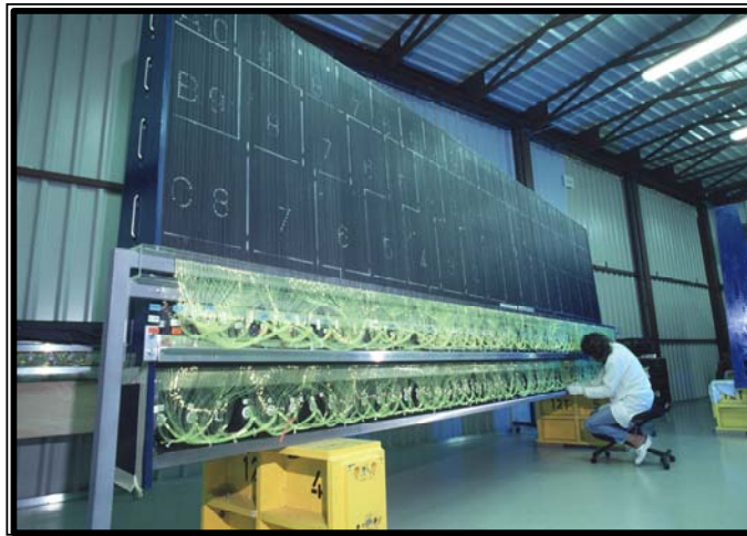
Figure 3. Fiber routing stage at end of instrumentation work on a module
